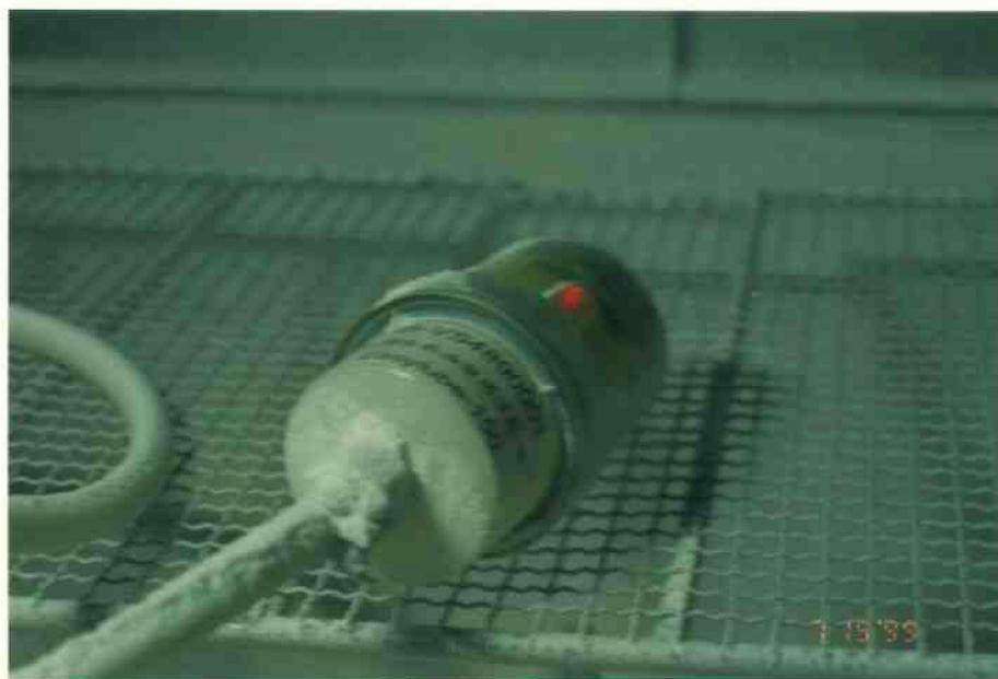
Fig.1 、 Installation of the dust test ( S/N:004007 )
